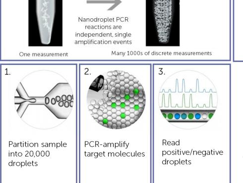
In consecutive steps, the rAAV sample dilution is partioned in about 20,000 droplets in a Droplet Generator (1), amplified in a Thermal Cycler (2) and positive and negative droplets are read on a QX200 Droplet Reader (3) followed by absolute quantification by Poisson
